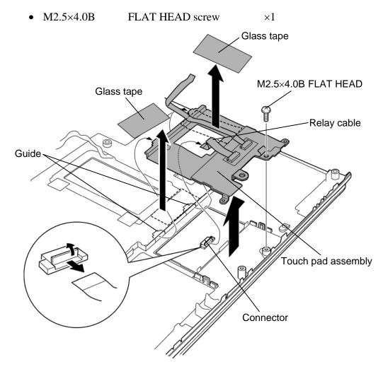
Figure 4-44 Removing the touch pad (1)
